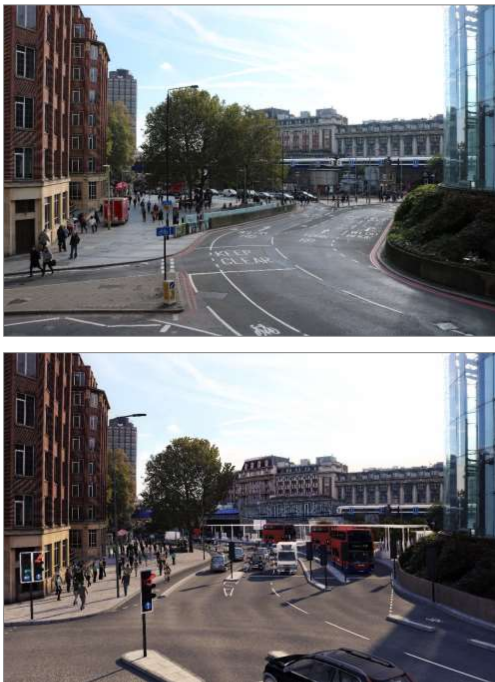
Figure 23: An example of an animation video produced using outputs from a Vissim model, with the existing image shown above and the scheme image shown below
