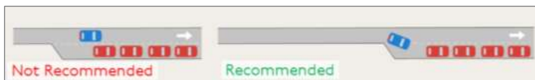
Figure 34: Side lane lengths. The Section on the left is too short.
