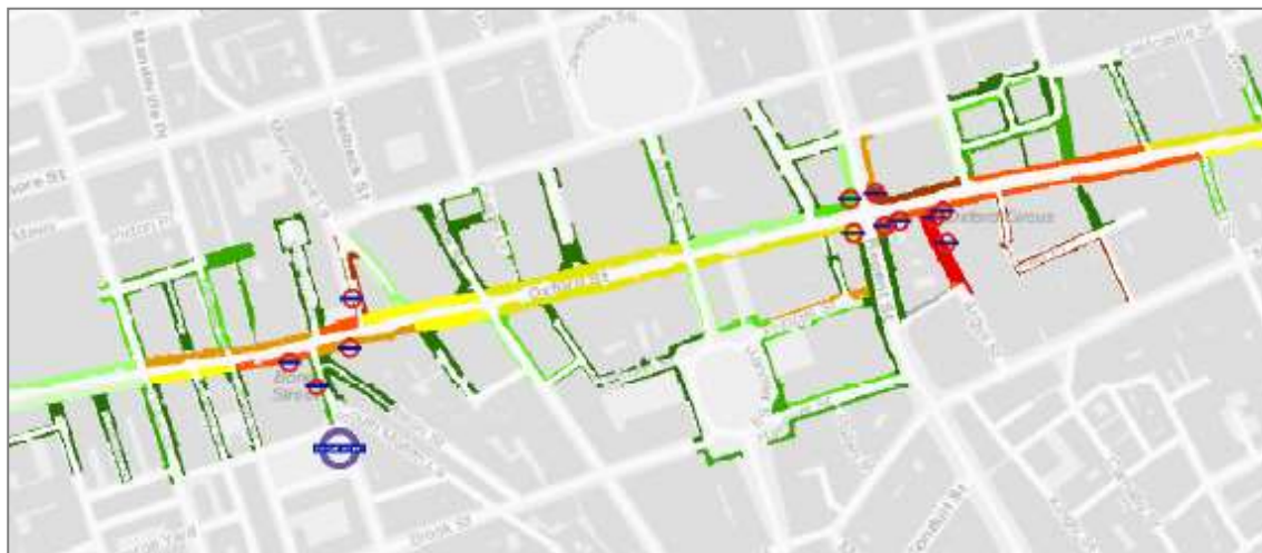
Figure 163: Pedestrian Comfort Levels applied to sections of footway
