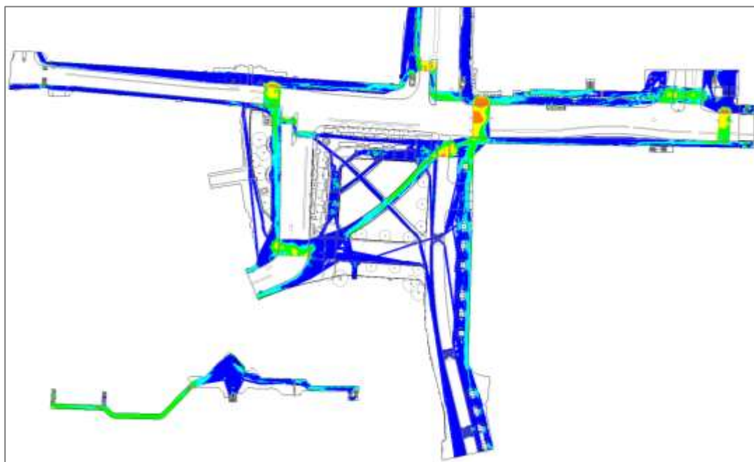
Figure 161: Heat map showing the Cumulative Mean Density for pedestrians across the peak 15 minutes, using Fruin's LoS for walkways
