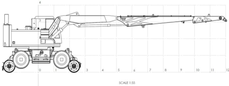
DX170 WITH 5.5M DIPPER + 1.5M DIPPER EXTENSION - BOOM CONFIGURATIONS
