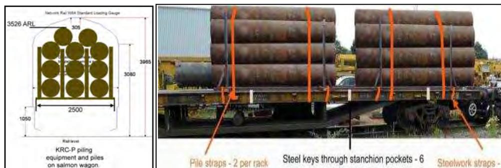
Figure 52: Securing and transportation of pile foundations
