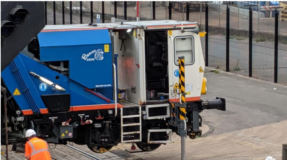
Arms beside each cab on each side stabilise the tamper whilst it is lifted off the ground. The arms at each end lift the machine.
