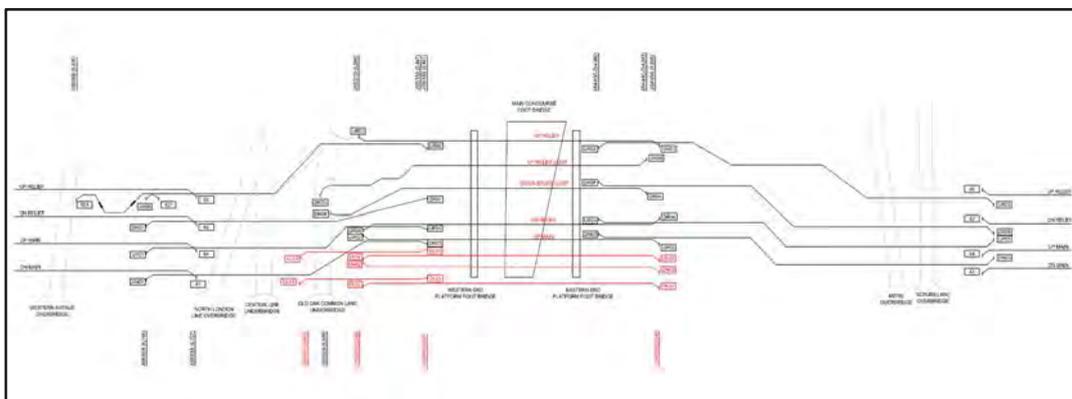
Figure 78: Station South wiring prior to Christmas 2026 blockade
