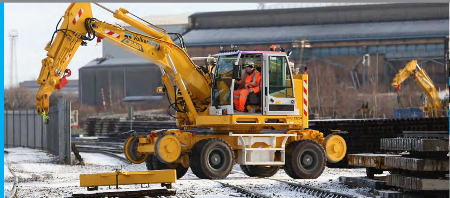
Rail mode – Level rail - Tool pin – unlocked - 0° - height
