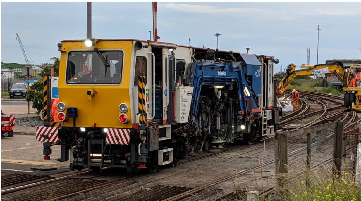
A Volker Rail lightweight tamper is seen on a level crossing at Newhaven Harbour during engineering work at Newhaven Marine aggregate sidings.
