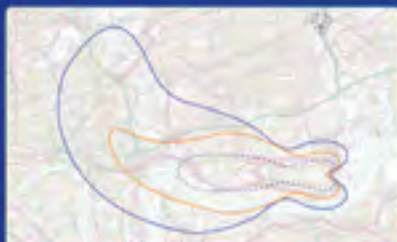
A comparison of the noise footprint of a new generation Embraer E175-42 with the footprint of an older generation Embraer E175. The new footprint is 10% smaller than the old footprint.
