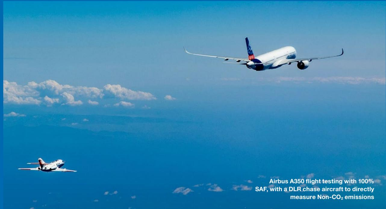
Airbus A350 flight testing with 100% SAF, with a DLR chase aircraft to directly measure Non-CO<sub>2</sub> emissions
