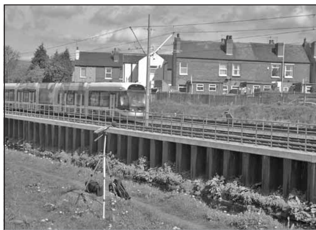
Fig. 8. A southbound NET tram travelling at 50 mph on ballasted track. Note the rail lines to the rear of the picture and the northbound tram track to the front
