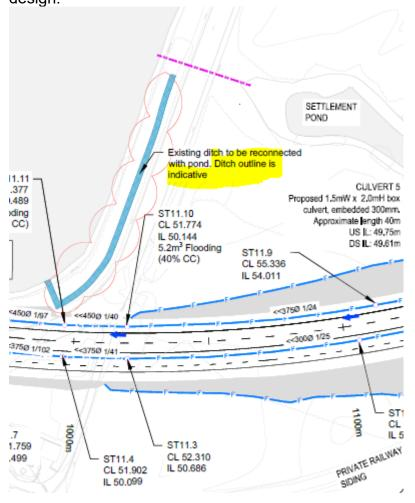
Entry points to swales etc – information required at detailed design. Design against blockage for inlets/outlets.
