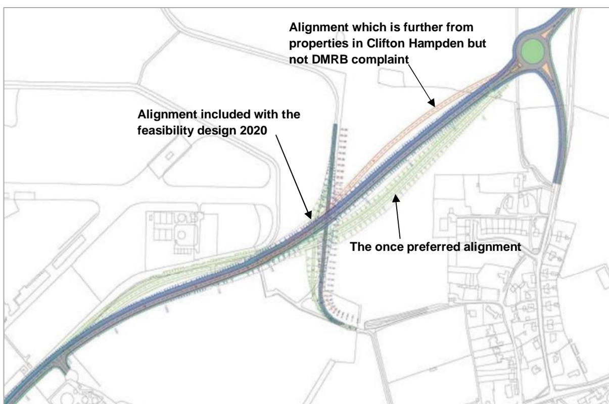
**Figure 3.15: Clifton Hampden Bypass alignment options (figure shows the once preferred 60 mph alignment in Green and a DMRB non-compliant alignment in red)**
