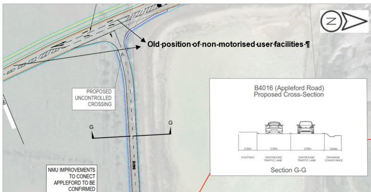
**Figure 3.10: Initial design for pedestrian facilities along the B4016 into Appleford**
