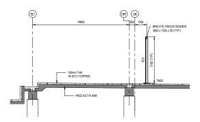
TEMPORARY NOISE BARRIER TYPICAL SECTION (LOOKING WEST)  $^{1:100}_{\phantom{000}}$
