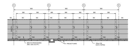
TEMPORARY NOISE WALL BARRIER TYPICAL ELEVATION (LOOKING NORTH)
