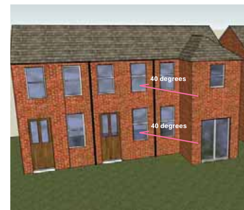
Fig 10.4 The 40 degree rule: The proposed extension should not project beyond the '40 degree line' (indicated by the dashed line) into the neighbours protected area
