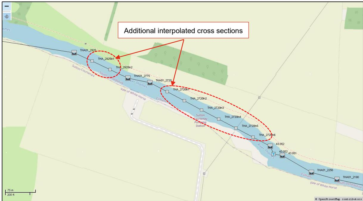
Figure 6 Interpolated cross sections added to 1D channel
