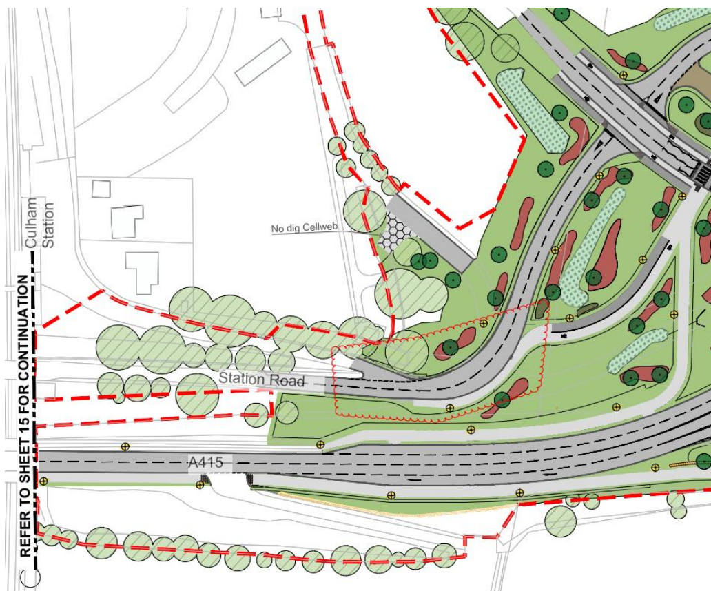
Figure 43 Proposed layout with shared use facility on the southern side of Station Road
