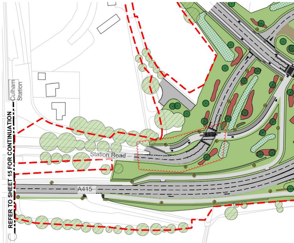
Figure 42 Previous proposed layout with segregated cycle track on northern side of Station Road
