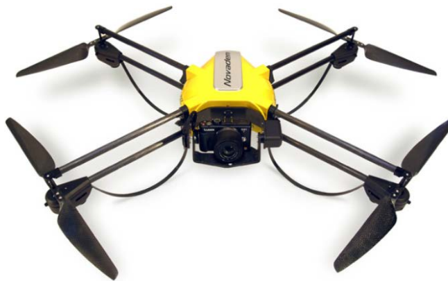
Figure 2: Example of a drone with camera mounted equipment to enable visual inspections without working from height
