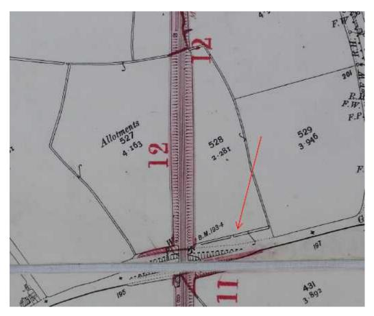
The arrow on the above plan points to a drain which is considered to be part of the highway, heading east from the underbridge on the north side of Pound Hill. Network Rail's view is that water drains from under the bridge, flows along this drain, and then flows north west, under the railway by way of a culvert, and then further west. This is in line with the general direction of flow of the drainage in the area.
