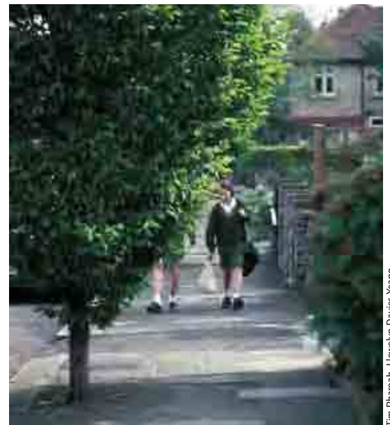
Figure 6.10 Poorly maintained tree obstructing the footway.
