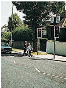
Additional signal heads may be employed at a signal-controlled crossing where this will improve driver awareness
