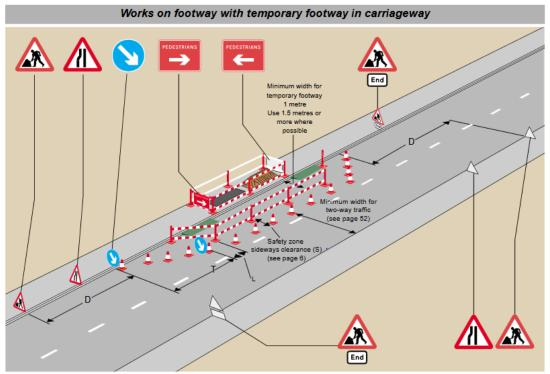
For numbers and size of cones, length of lead in taper (T) and dimensions 'D', 'L' and 'S' see table inside back cover. Information boards should also be displayed (although omitted here for clarity). See page 20.
