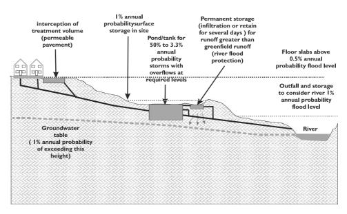
Figure 4.7 Illustrative schematic of a storage layout (adapted from Kellagher, 2004)
