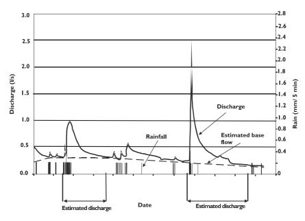
Figure 9.2.4 Example hydrograph from outfall of pervious pavement at Wheatley MSA
