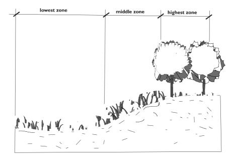
Figure 9.7.9 Planting zones for swales (Richman et al, 1998)
