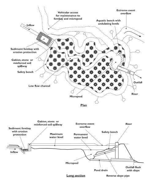
Figure 9.11.11 Example details of an extended detention basin (Highways Agency et al, 2001)
