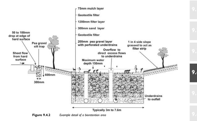
Various geotextile filters can be provided within the construction to stop the migration of fines between layers and to trap hydrocarbons. A shallow geotextile provided at 150 mm depth into the soil filter is useful to keep clogging and the retention of hydrocarbons as high in the system as possible to aid maintenance.
