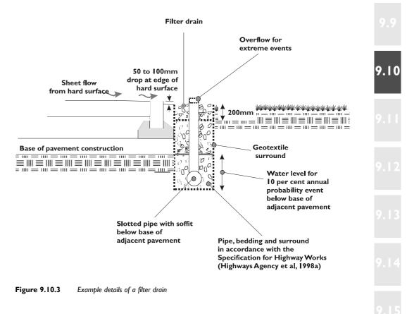
A geotextile should be provided around the outside of the filter drain. If a geotextile is placed over the top of the filter material at 200 mm depth it will collect sediment and prevent blockage of the whole depth of filter, thus minimising the volume of material requiring replacement when the filter eventually clogs.
