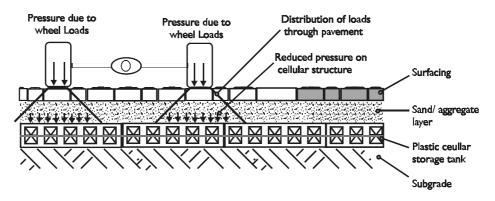
Figure 9.13.6 Spread of load below a wheel
