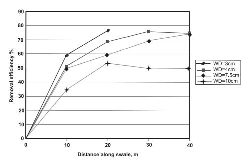
Figure 9.7.3 Effect of water depth and swale length on TSS removal efficiency (Walsh et al, 1997)
