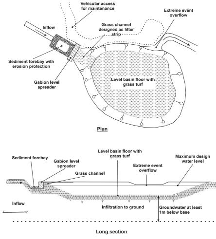
Figure 9.9.2Example details of an infiltration basin
