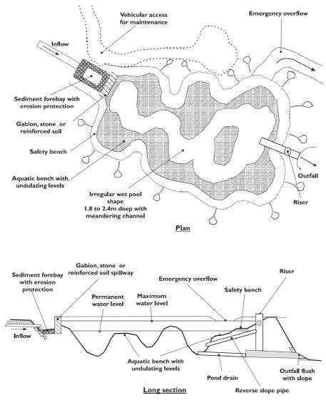
Figure 9.11.6 Example details of a wet pond
