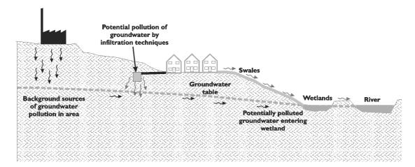
Figure 3.4 Example of a conceptual model for a SUDS scheme
