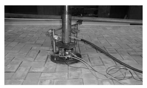
Figure 9.13.7 Testing of a full-scale pavement incorporating a plastic cellular sub-base replacement system
