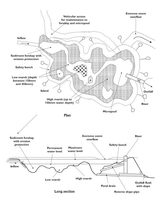
Figure 9.12.2 Example details of a wetland for stormwater treatment (Maryland Department of the Environment, 2000)
