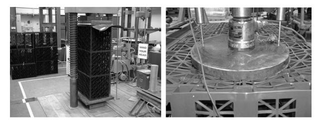
Figure 9.13.2 Compression test configurations on plastic cellular structures
