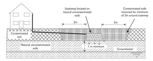
Figure 2.4 Example installation of an infiltration system on a contaminated site
