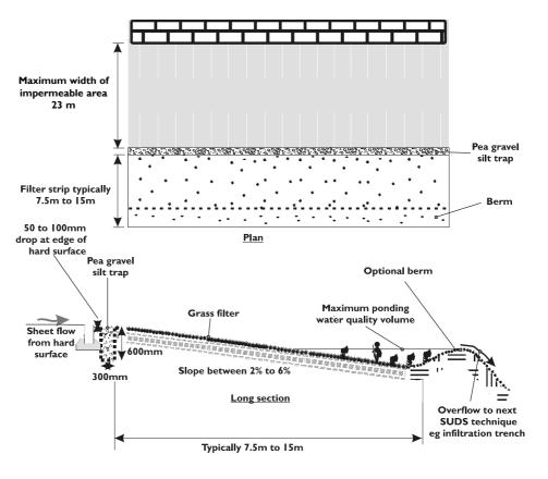
Figure 9.6.2 Example details of a filter strip
