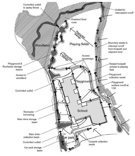
Figure A4.8 Plan of drainage system
