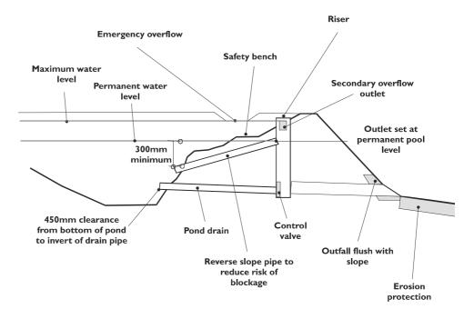
Figure 9.11.8 Example outlet detail for ponds (Minnesota Metropolitan Council, 2001)
