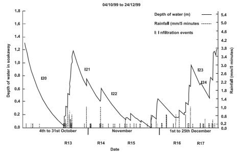
Figure 9.8.4 Response of soakaway to rainfall events (Abbott et al, 2000)
