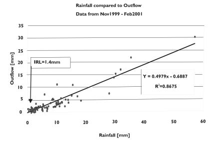
Figure 9.10.2 Rainfall compared to outfall from a filter drain (Jefferies, 2001)
