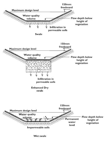
Figure 9.7.2 Types of swale (Claytor and Schueler, 1996)
