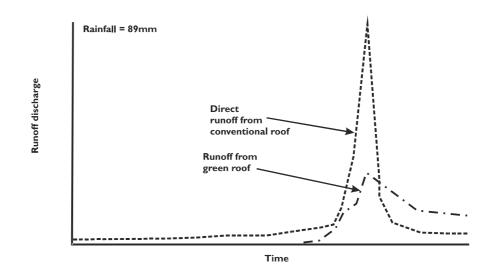
Figure 9.3.3 Runoff hydrograph from a green roof (New Jersey Department of Environmental Protection, 2000)
