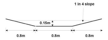
Figure A2.3 Section of bioretention area
