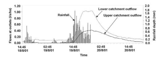
Figure A4.5 Outflow hydrograph for a typical rainfall event (Schluter, Spitzer and Jefferies, 2000)
