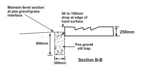
Figure 9.4.3 Diversion structures to bioretention areas (Claytor and Schueler, 1996)
