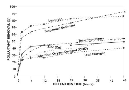
Figure 9.11.2 Removal rate versus detention time for wetlands (Grizzard et al, 1986, quoted from Schueler 2000b)
