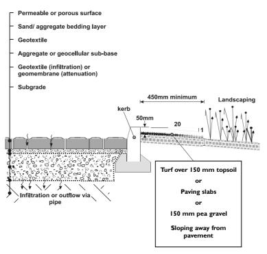
Figure 9.2.5 Pervious pavement details
