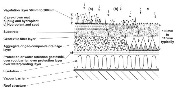
Figure 9.3.5 Example details of a green roof (Tarr, 2002)
