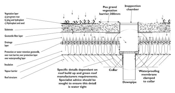
Figure 9.3.6 Example detail of outlet from green roof
