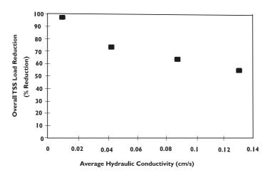
Figure 9.5.3 TSS reduction and hydraulic conductivity (Tenney et al, 1995)
