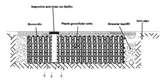
Figure 9.8.2 Example soakaway construction
