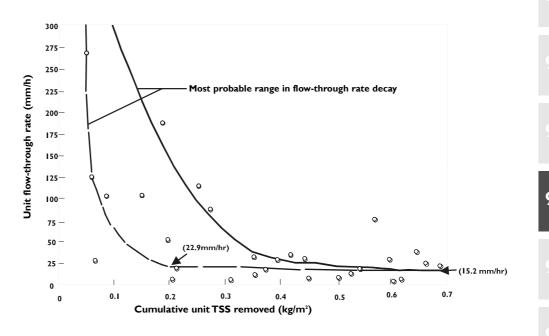
Figure 9.5.4 Flow rate versus cumulative TSS removed (Urbonas, 2000)
