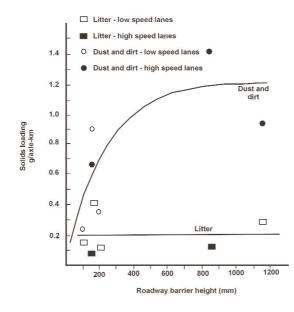
Figure 3.2 Effect of kerb height on particle loading of street surface (Novotny and Olem, 1994)
