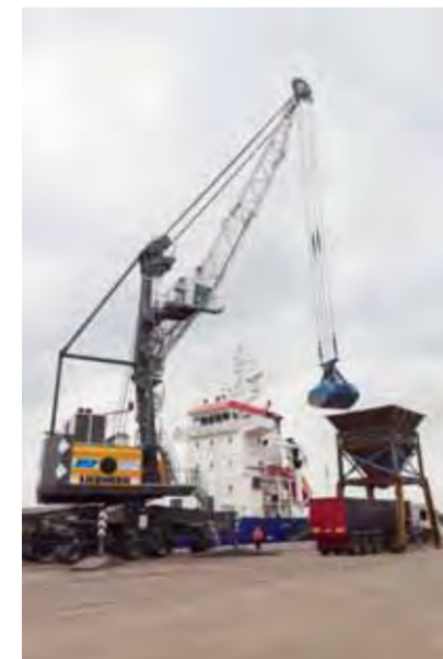
LHM 180 mobile harbour crane with a height of 48.8m at the Port of Newport
