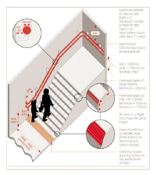
Tread depth or going should be **300mm** deep (approximately the length of a size 9 shoe), never less than **250mm** and the nose of the step should be rounded (**6mm** radius) without any overhang. People with walking difficulties often pull their feet up the face of the riser; any overhang will catch their foot.
