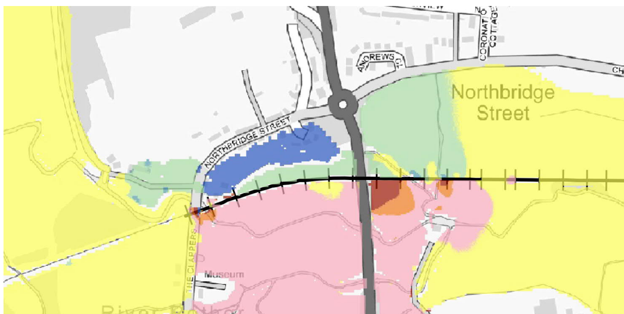
Figure 6.4a: Extract from Capita Flood Mapping 2020 – Figure 4-9 1% AEP Design Flood Event with 105% allowance for climate change - Difference in 'With Railway' and Baseline predicted Maximum Water Level
