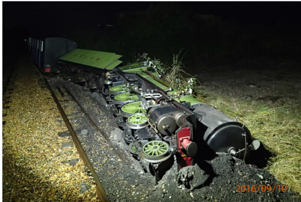
Romney Hythe and Dymchurch locomotive Number 1 'Green Goddess' lying on its side after the accident
