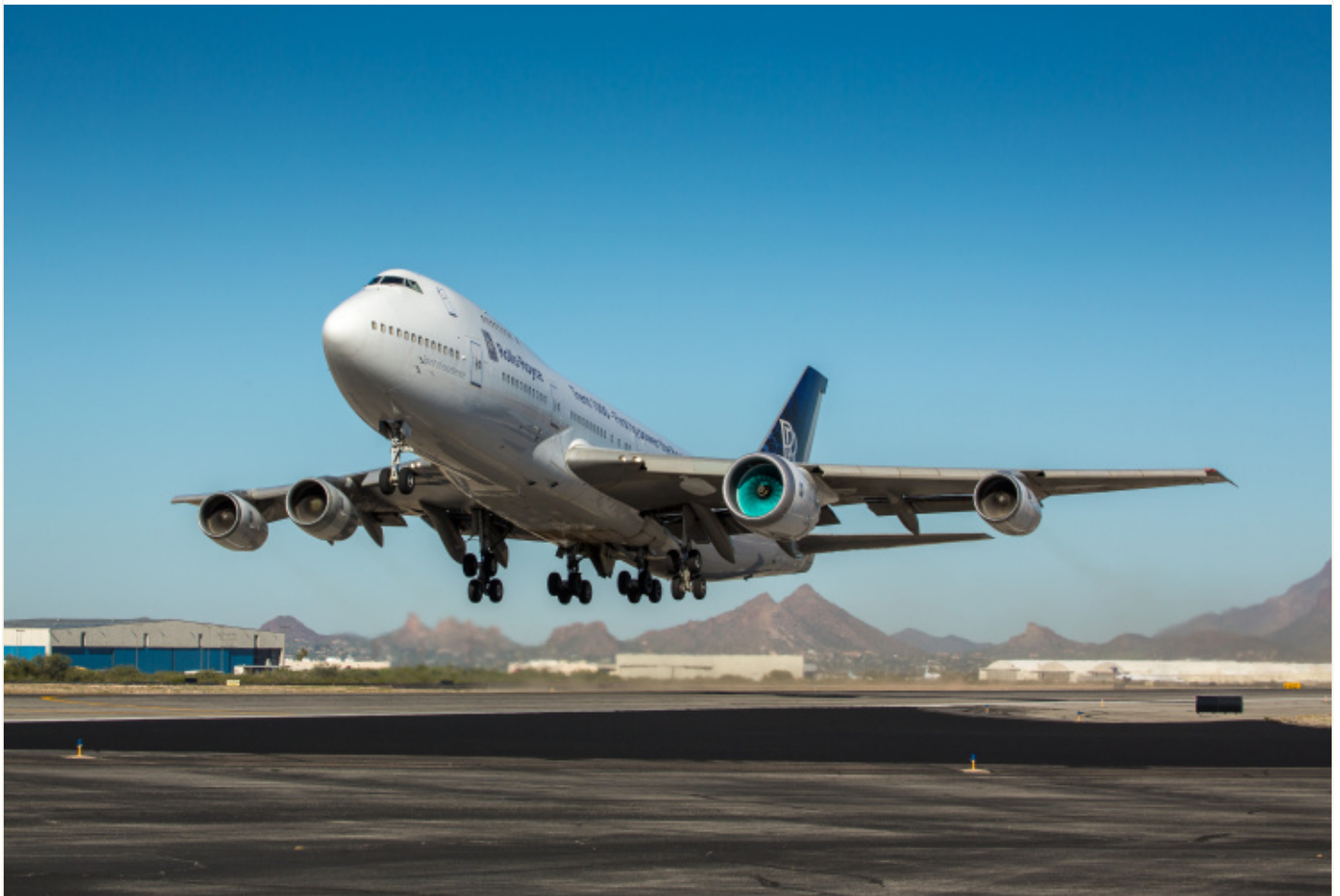
Flight-testing blue composite fan-blades, on right of image (courtesy Rolls-Royce)
