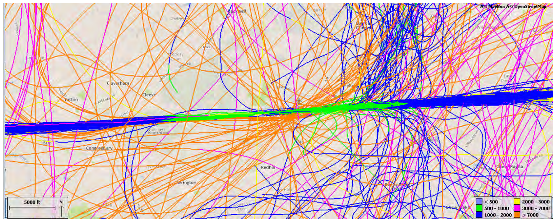
Figure 7 Flight tracks and AGL ft for aircraft arrivals over the SAC
