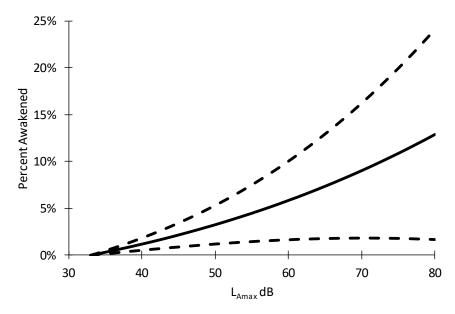
**Figure 7.** The unadjusted probability of an additional awakening induced by aircraft noise depending on indoor maximum sound pressure level  $L_{Amax}$  (slow time weighting) for PHL International Airport. Dashed lines indicate 95% confidence intervals.
