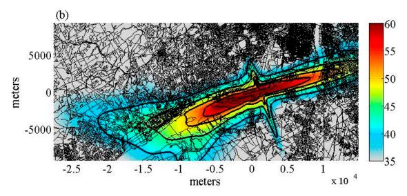
**Figure 2.** Average  $L_{night}$  contours for (a) East flow configuration (13.2% of modeled nights) and (b) West flow configuration (86.3% of modeled nights). The contour lines shown are the 40, 45, 50, and 55 dBA  $L_{night}$  contours.
