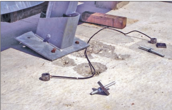
Figure 5.18 Failed restraint support – bolt failure (after impact)
