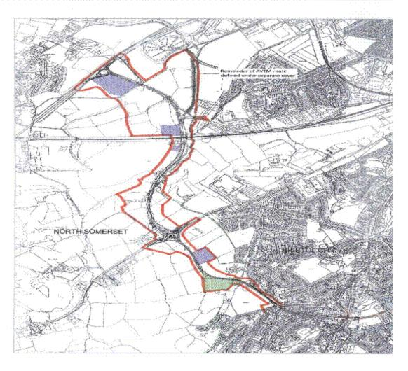
1. 13/P/1204/F2 SOUTH BRISTOL LINK: PROPOSED HIGHWAY AND BUS ONLY LINK INCLUDING BRIDGES, STRUCTURES, CONSTRUCTION COMPOUNDS, DRAINAGE A LANDSCAPING; TRAFFIC SIGNS, LIGHTING AND BUS SHELTERS; SHARED CYCLEY AND FOOTWAY; WORKS TO EXISTING HIGHWAYS AND PROVISION OF REPLACEMENT HIGHRIDGE COMMON LAND, ON LAND BETWEEN THE A370 LONG ASHTON BYPAS NORTH SOMERSET AND THE CATER ROAD ROUNDABOUT IN HARTCLIFFE, SOUTH
