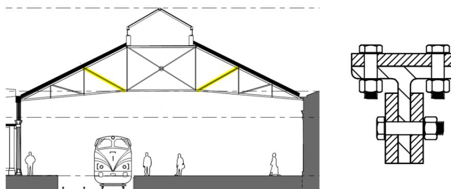
Figure 5.1.9.2a: Strengthening detail to diagonal elements
