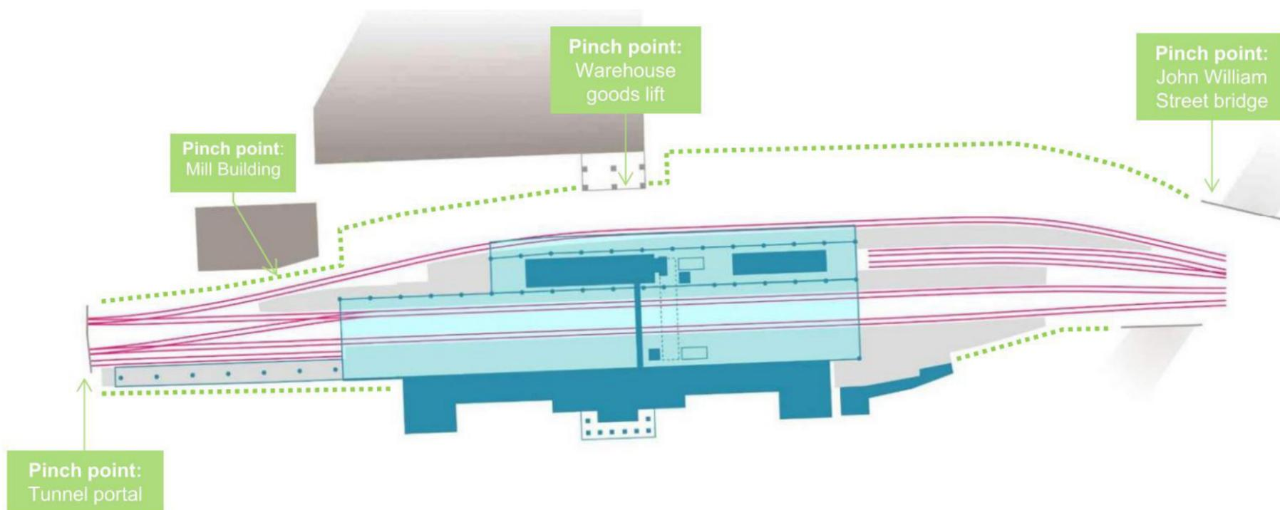
Figure 4.1.2c: Site boundary with 'pinch points'
