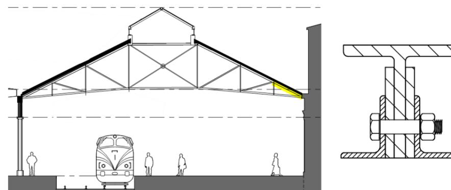
Figure 5.1.9.2c: Strengthening detail to top boom
