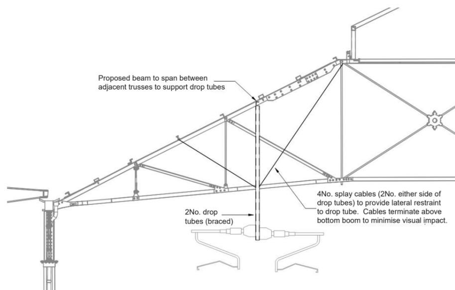
Figure 5.1.7a: Proposed OLE installation
