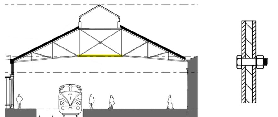
Figure 5.1.9.2b: Strengthening detail to bottom boom of 6No. trusses at Manchester end of Roof A
