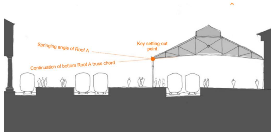
Figure 4.7b: Setting out lines derived from Roof A
