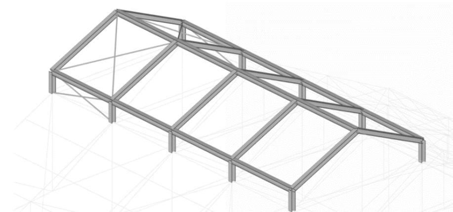
Figure 5.1.9.3a: Proposed lantern structure
