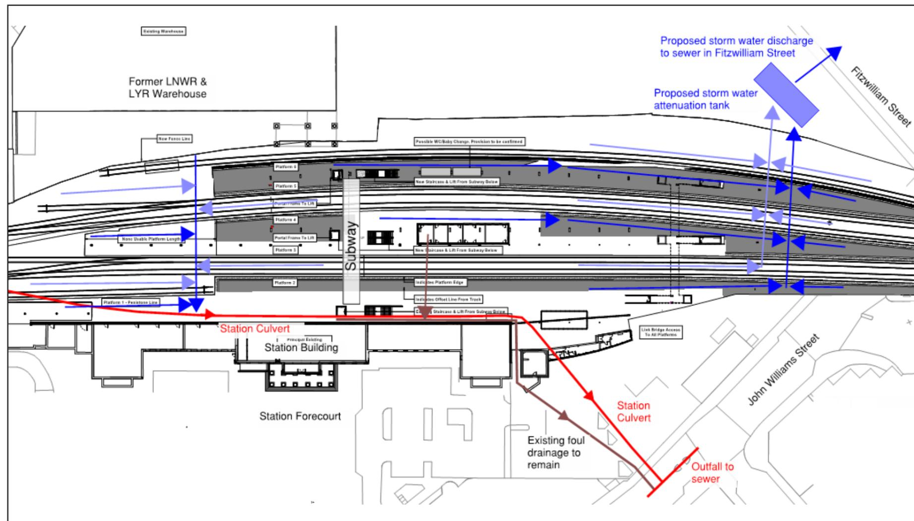
Figure 5.4.8.2a: Proposed drainage systems
