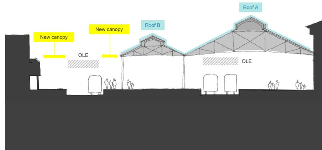
Figure 4.1.5d: Option 1 - new canopy coverage required (section)
