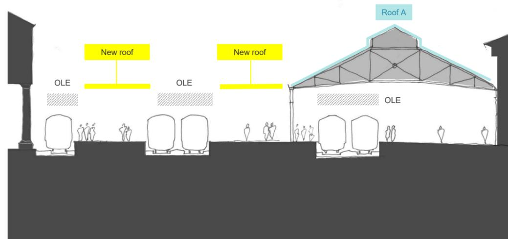
Figure 4.1.4d: Option 0 - new canopy coverage required (section)
