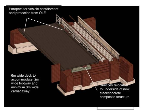
Figure 27 Sheepwash Bridge, isometric view on proposed decks 4 and 5
