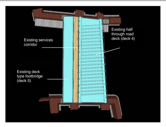
Figure 24 Sheepwash Bridge, plan on existing decks 4 and 5
