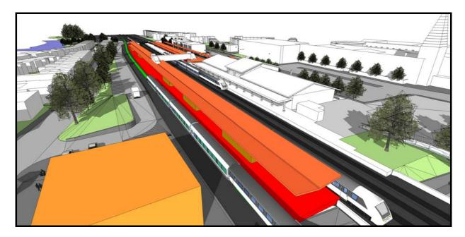
Figure 43 Platform 4/5 Canopies Proposal isometric
