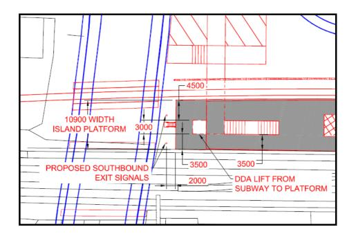
Figure 3 Lineside access, South end of new island platform
