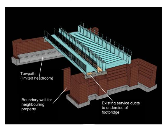
Figure 25 Sheepwash Bridge, isometric view on existing decks 4 and 5
