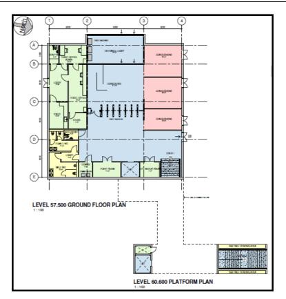
Figure 34 Western Entrance, Proposed Floor Plans – Pedestrian 'surface' level
