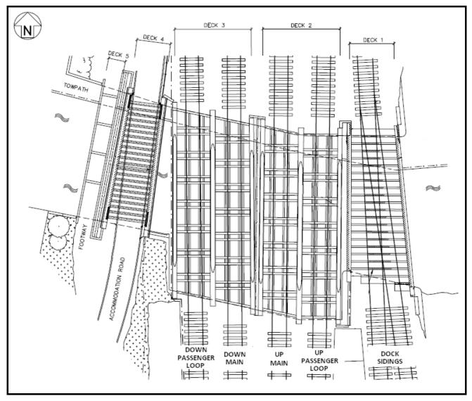
Figure 18 Plan on existing Sheepwash bridge crossing
