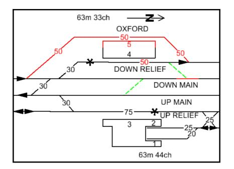
Figure 40 Schematic Phase 2 Track Layout
