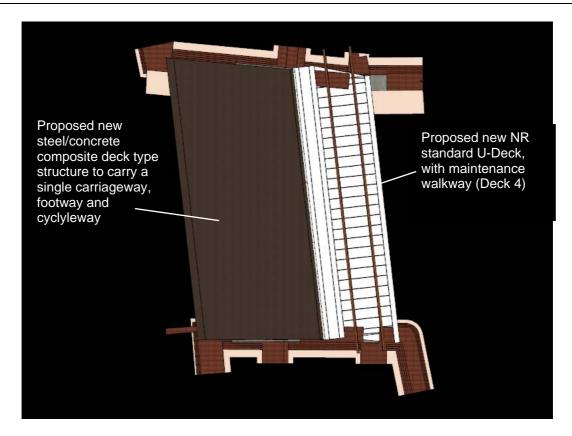
Figure 26 Sheepwash Bridge, plan on proposed decks 4 and 5
