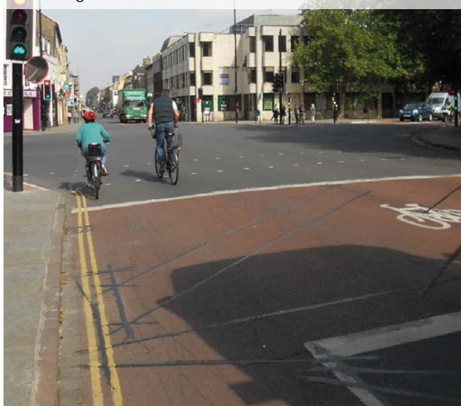
Figure 10.23 'Cycle Filter' signal used for an early release, Cambridge
