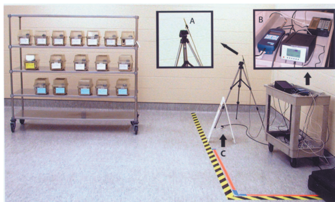
FIGURE 1. Photograph of noise and vibration monitoring equipment located in one of the animal housing rooms. Insert A is an enlarged photograph of the sound microphone sensor positioned on top of a tripod stand. Insert B is an enlarged photograph of the control and recording equipment positioned on top of the cart. Arrow C indicates the position of the vibration sensor glued to the floor of the room.
