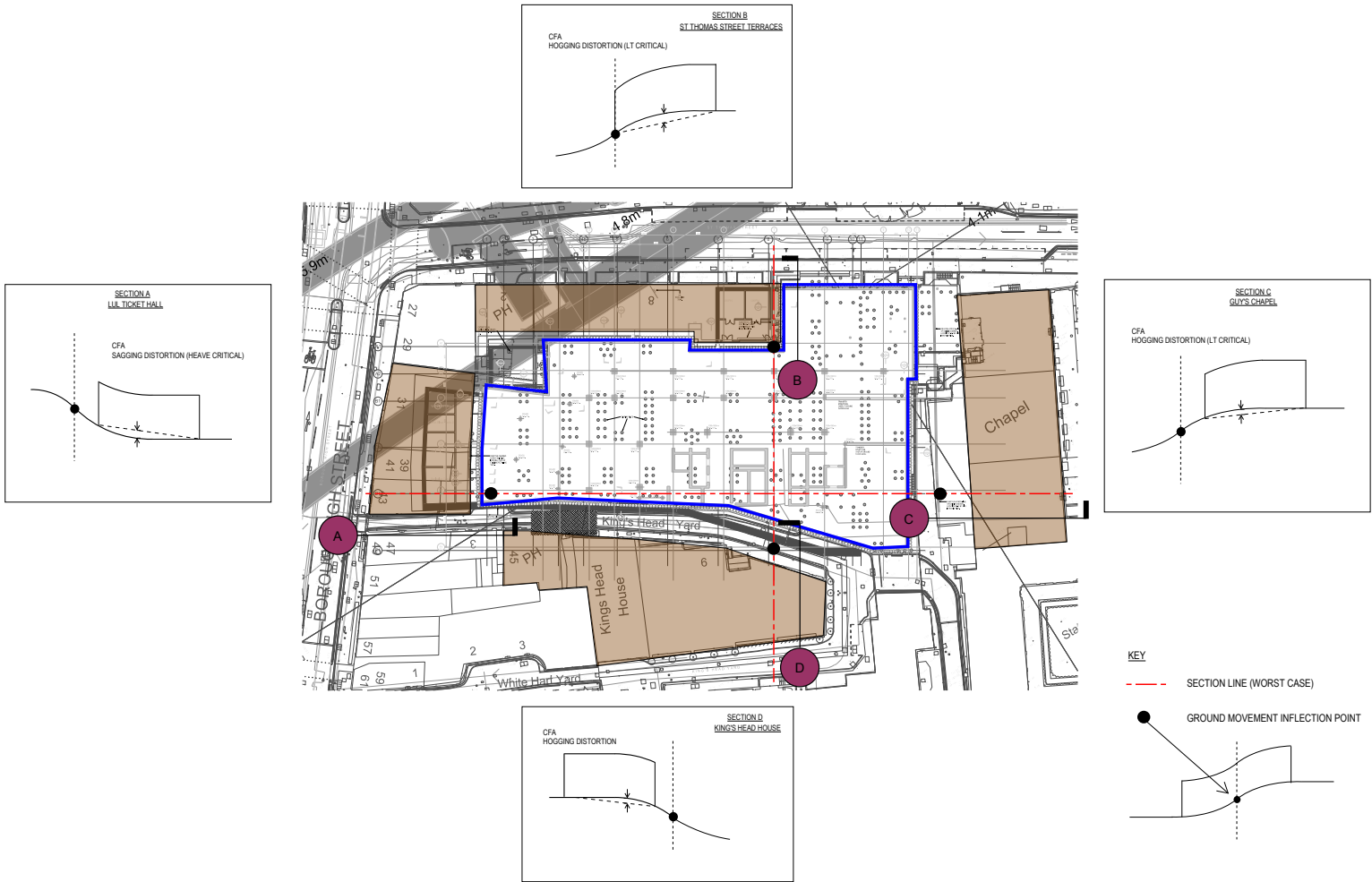
Figure 10.2 Adjacent buildings behaviour due to settlement plot of NCC development
