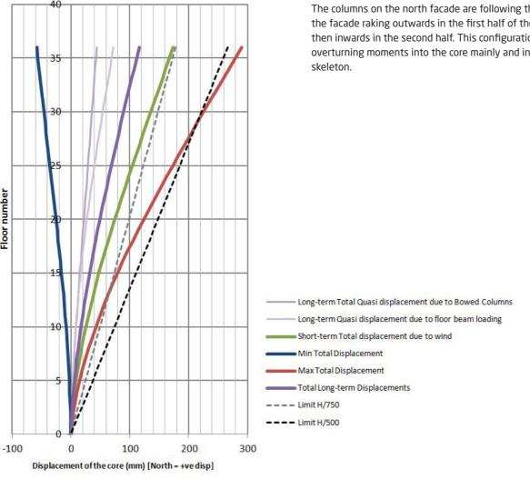
Figure 8.6 Lateral movements of the core
