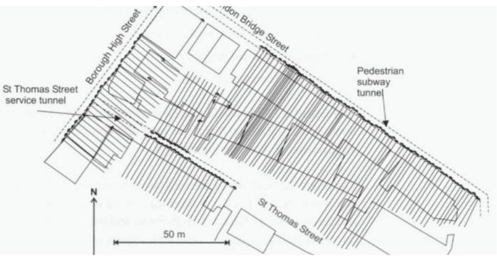
Figure 6.5 Plan of space with TAM locations in relation to the proposed site
