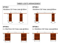
NOTE: TIMBER JOISTS SPACING DRIVEN BY PLYWOOD FLOORING STA
