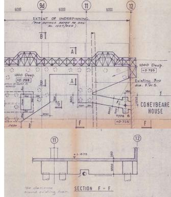
Figure 6.2 Sewer location below Keats House as shown on Engineer's plan section F-F
