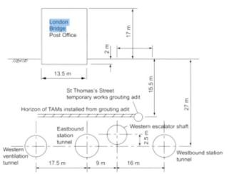
Figure 6.7 Compensation grouting - section through St. Thomas street
