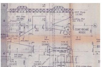
Figure 7.6 Record drawing showing existing foundations
