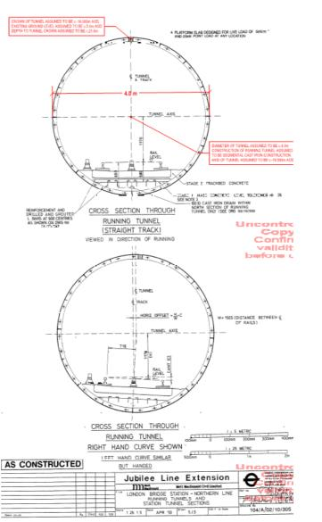
Figure 6.4 Northern Line Tunnel
