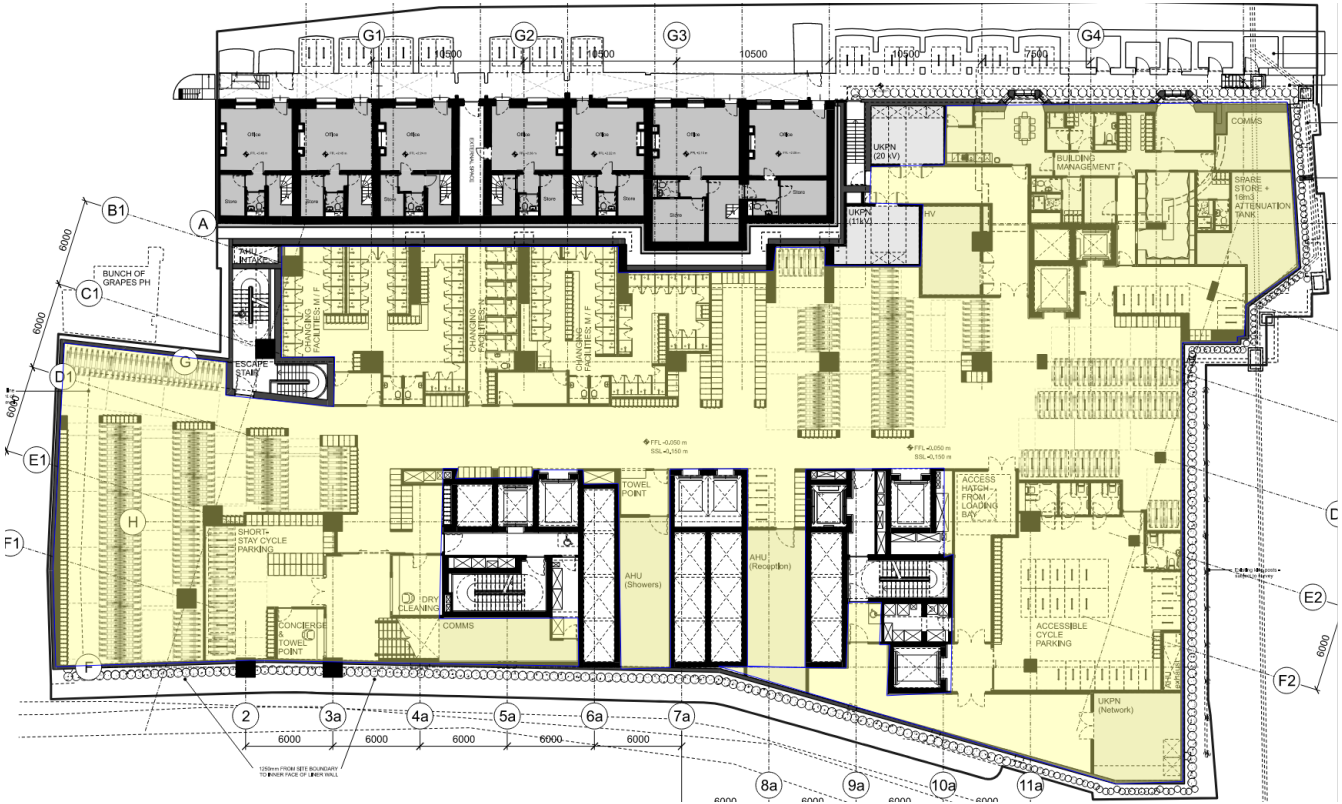
Image 03: Areas served by Louvre Intake and Exhaust in B1.
