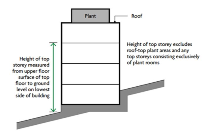
Diagram measuring height of building for planning gateway one shows that the height should be measured from the upper floor surface of the top floor to ground level on the lowest side of the building. Excluding roof top plant areas and any top storeys consisting exclusively of plant rooms.
