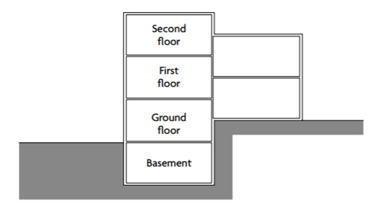
Diagram showing that basement storeys should not be counted when counting storeys, and where the number of storeys varies from ground level they should be counted from the lowest external ground level.
