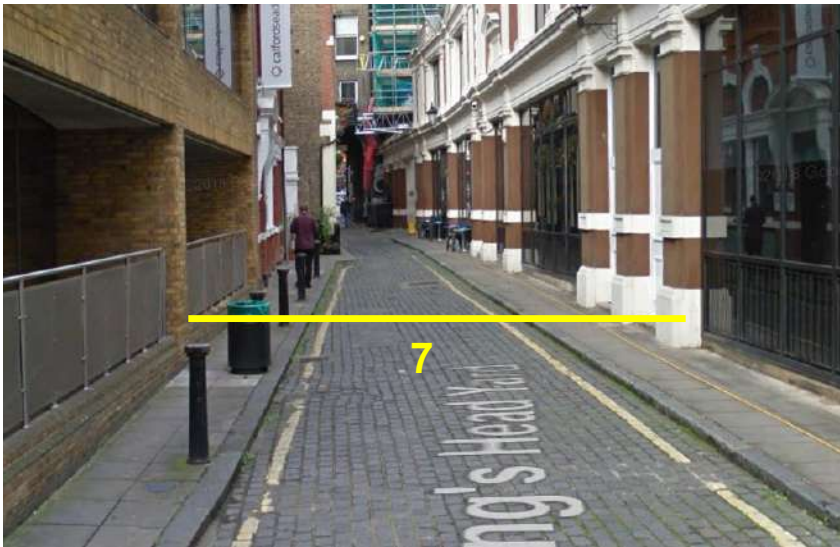
Location 7 Total width: 5.70m (bollard) (full street width-shared space) Effective width: 4.4m
