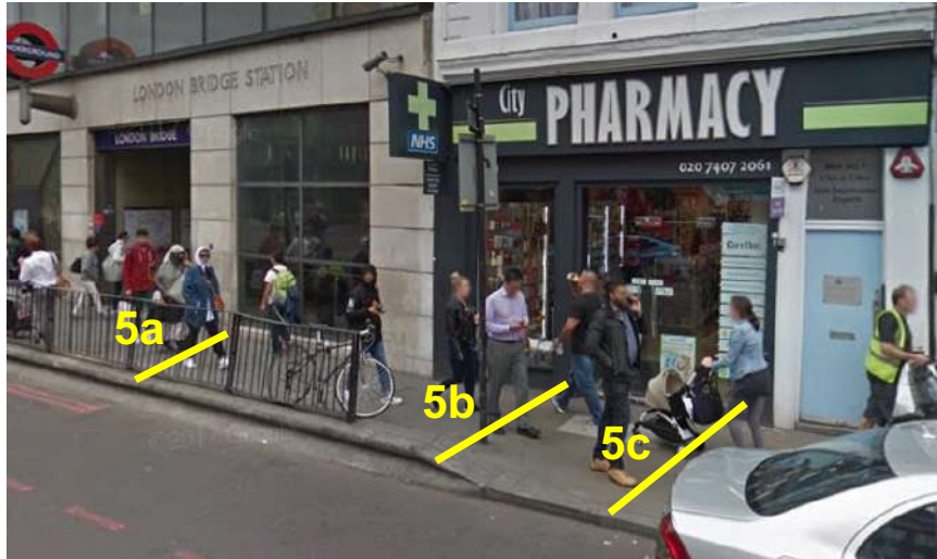
Location 5 5a Total width: 3.40m (railing) Effective width: 2.40m 5b Total width: 3.10m (sign post and railing) Effective width: 1.80m 5c Total width: 2.90m Effective width: 2.50m
