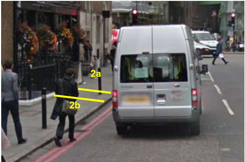
Location 2 2a Total width: 1.90m (bollard) Effective width: 0.90m 2b Total width: 2.0m Effective width: 1.60m
