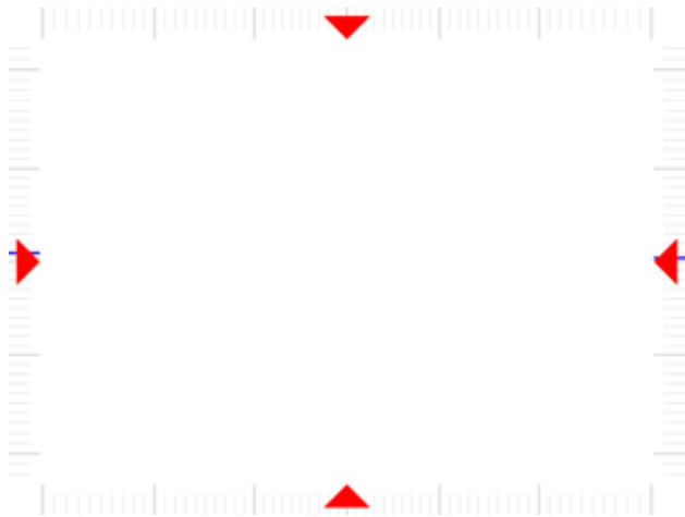
Sample graticule showing optical axis markers
