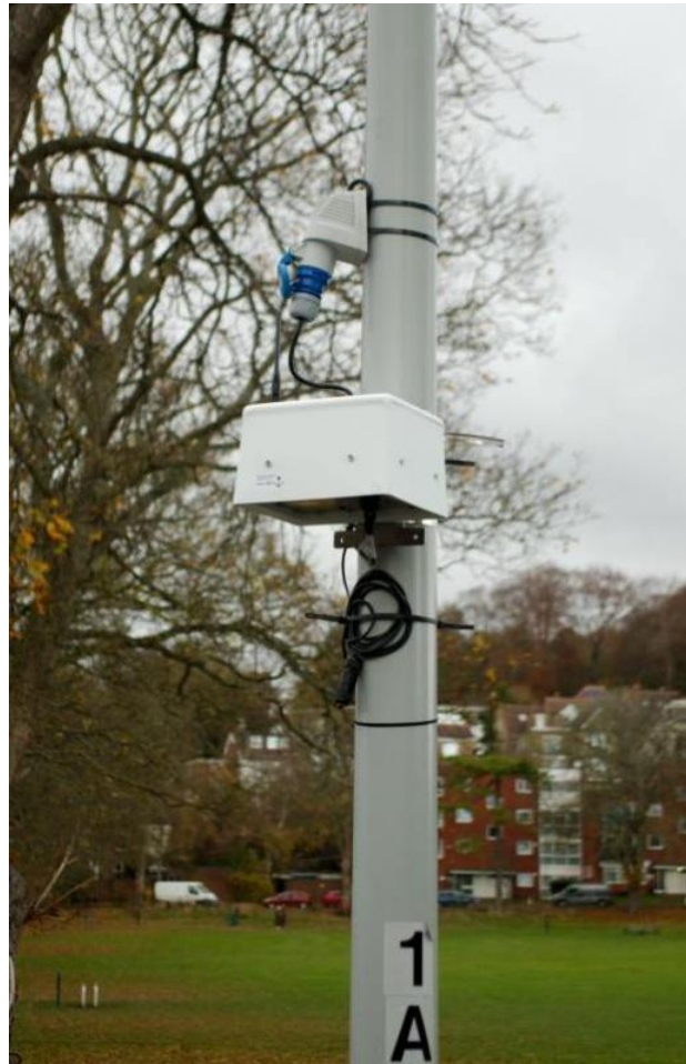
Figure 1 – One of five newly installed indicative air pollution monitors
