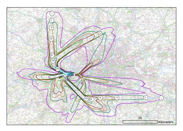
Figure 20: Overflight contours, 60° cone, to 7,000 feet
