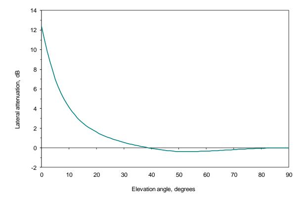
Figure 10: Attenuation of noise from aircraft with wing-mounted engines vs elevation angle (source, SAE International AIR-5662)
