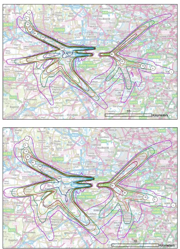
Figure 14: Overflight contours for a typical summer day at Heathrow Airport, to 4,000 feet – departures only (60° and 48.5° cones respectively)
