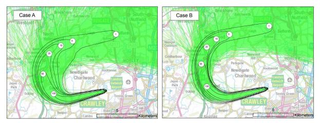
Figure 18: Overflight contours, 48.5° cone (up to 4,000 ft altitude)
