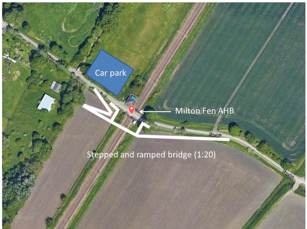
Figure 32 Downgrade crossing to UWC and replace with pedestrian bridge and car park
