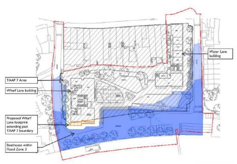
Figure 17. Flood Zone and TAAP Overlay Diagram
