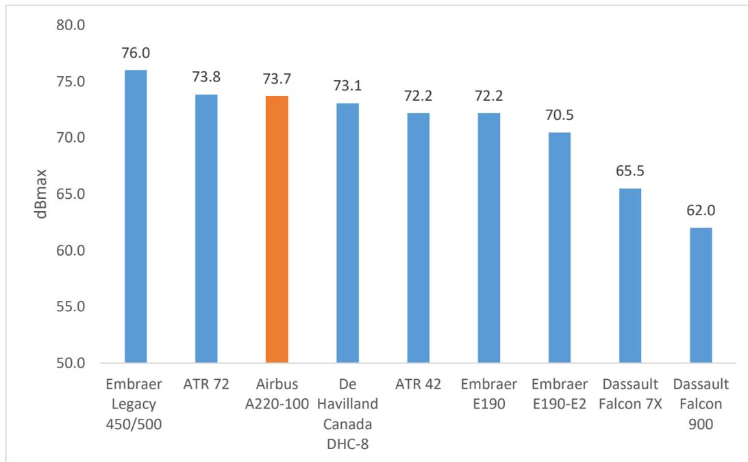
**Table 5.** Ranking of the noisiest aircraft during overflight. The orange bar is the new generation Airbus A220-100, which is the third loudest aircraft overall.
