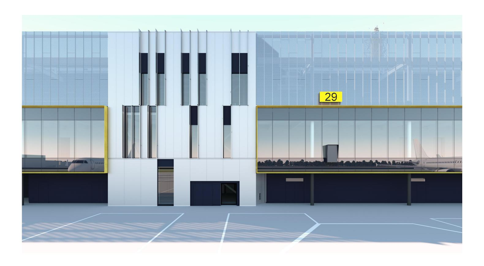
Figure 4.0.3: New Eastern Pier partial elevation - Proposed scheme without mesh to the solid areas of the façade and with exposed, enhanced composite panelling. Mesh is retained where the L20 roof plant areas, as per the approved scheme treatment.
