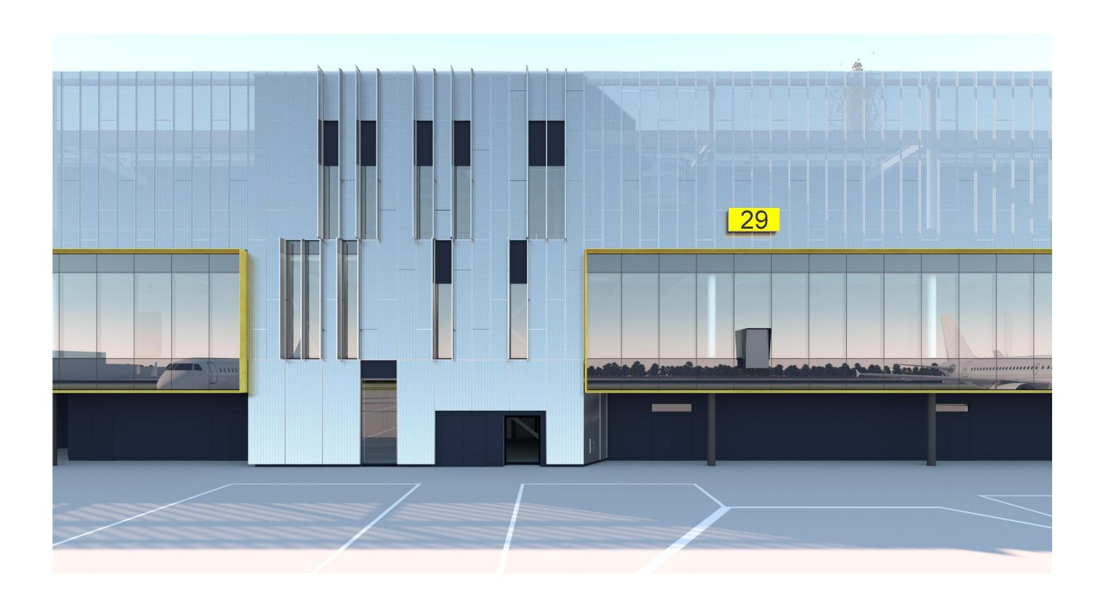
Figure 4.0.2: New Eastern Pier partial elevation - Approved scheme with expanded metal mesh over composite panelling.
