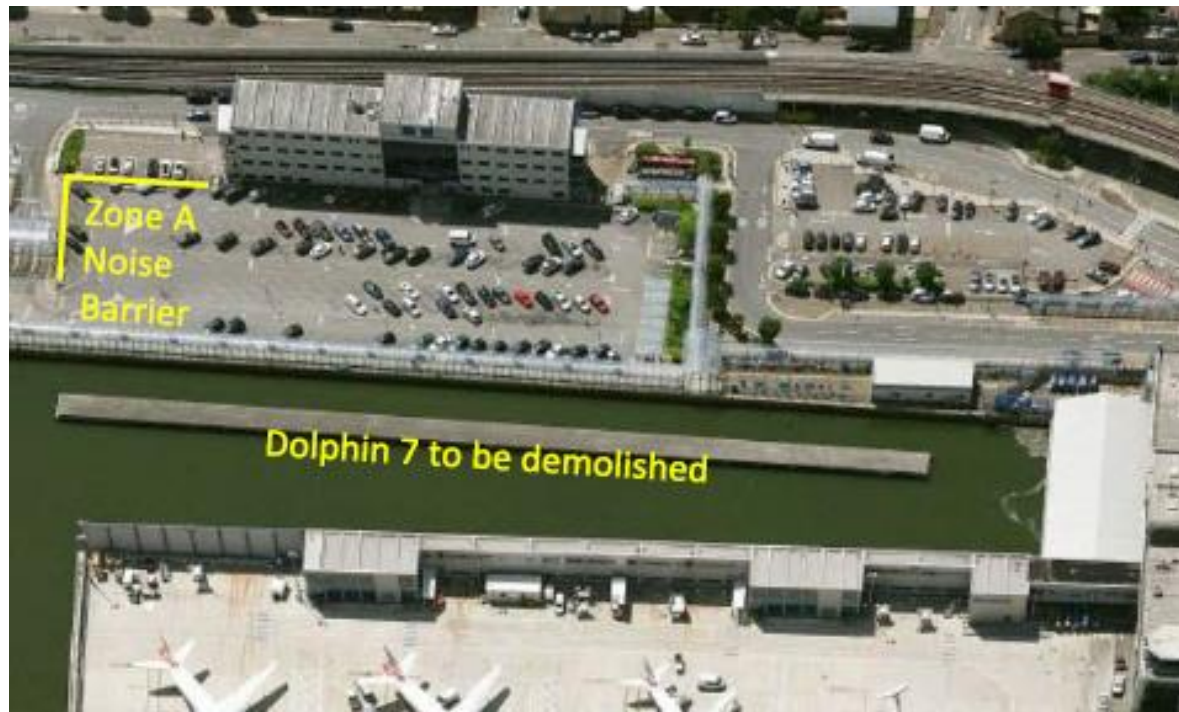
Figure 2: Extent of Construction Noise Barrier to be installed prior to commencing demolition of Dolphin 7
