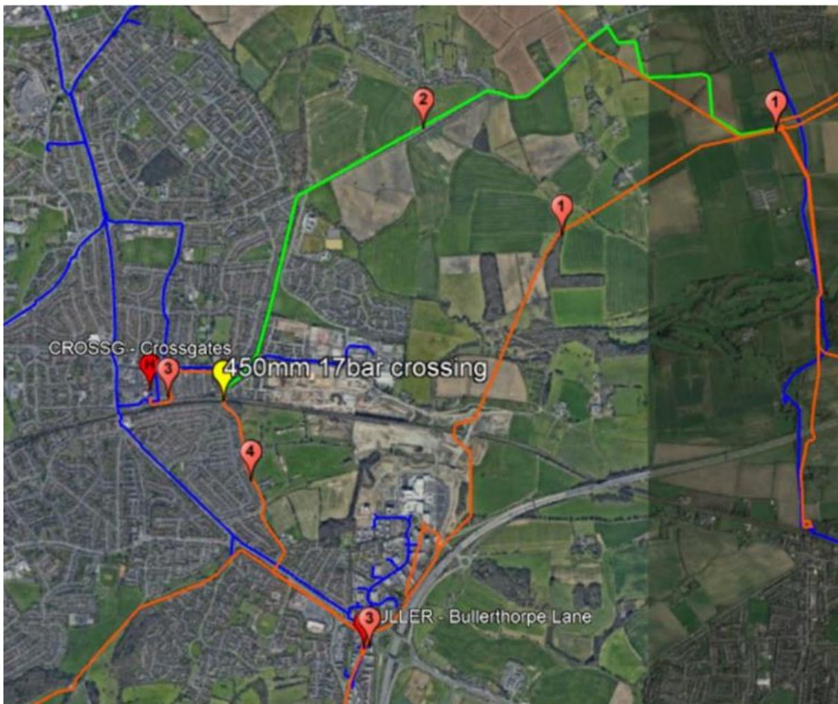
option 3. Downrating of 38bar into Leeds (1) removes the needs for Bullerthorpe Lane PRS, this site can be decommissioned and removed (3). IP reinforcement into Crossgate (2) removes the need for Crossgates 19-2bar PRS, this site can be decommissioned and replaced with 6.9-2bar district governor.
