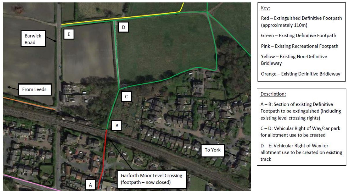
Figure 33 - Schematic of the Garforth Moor Level Crossing proposals
