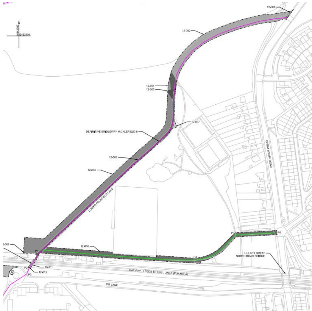
Figure 30 - Proposed footpath (or bridleway) between Lower Peckfield Lane and Great North Road, upgrade to Lower Peckfield Lane, parking/turning area and existing level crossing locations
