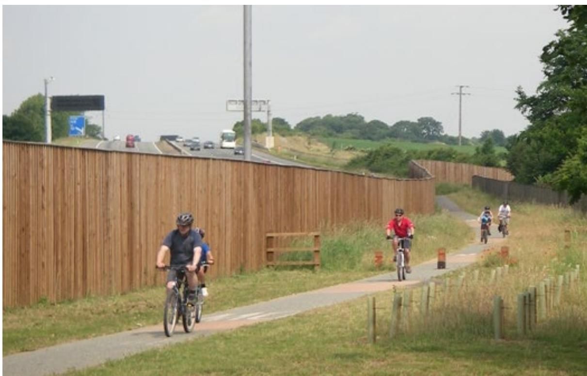
Figure 31: 3.0m Two-way Cycle Track with Barrier Layout
