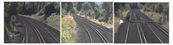
11.12 The train sounds its horn at the stage shown in the first photograph, which would have been heard by the ramblers before they crossed the railway at the crossing, around the bend. Approximately 5 seconds later the driver sees the ramblers on the crossing. Only 4 seconds from the crossing, the rambler (right) is shown to sprint over the lines despite seeing the fast-oncoming train and clears the train less than 1 second from being struck.
